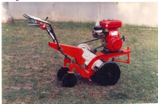
Figure 2: Prototype of Power tiller
